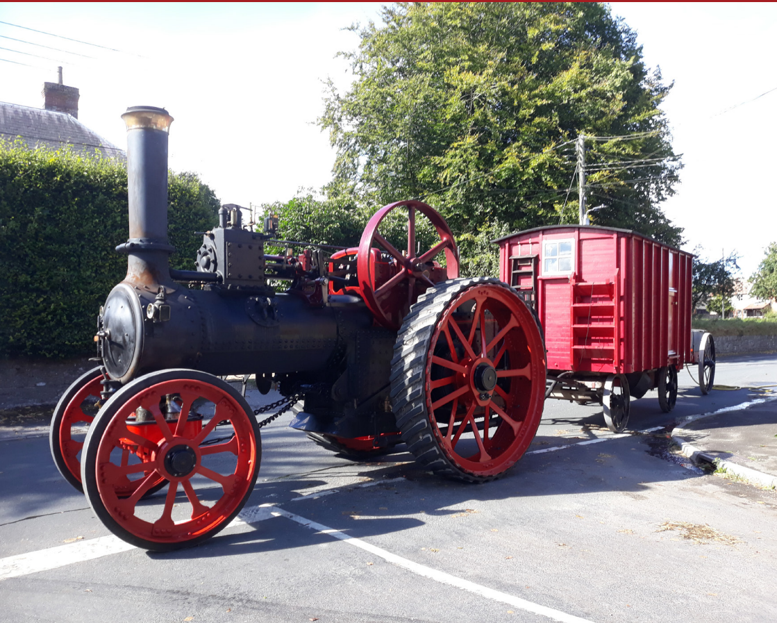
1913 Marshall 8 HP Steam Powered Traction Engine topping up with water in Church Street early this month
